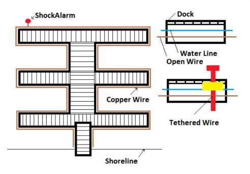
Improper Electrical Ground Detection
